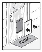
An additional closing panel (sold separately) can be used on the exterior frame of the Extreme Weather Pet Door™ for improved weather resistance. See "Replacement Parts and Accessories" on page 10.
