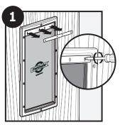
To Replace vinyl flap, remove flap screws and flap support from top of pet door frame.
